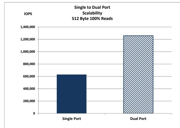
Figure 2. Scalability Across Ports for the QLE2672 Adapter
