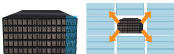
Figure 4. Expandable Centralized Switching Topology
